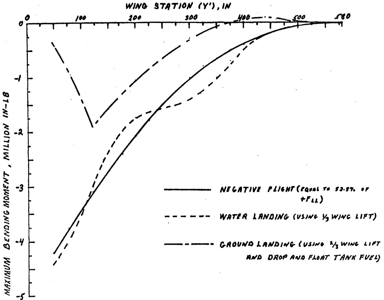
Fig. A-2--Comparison of negative bending moments.
