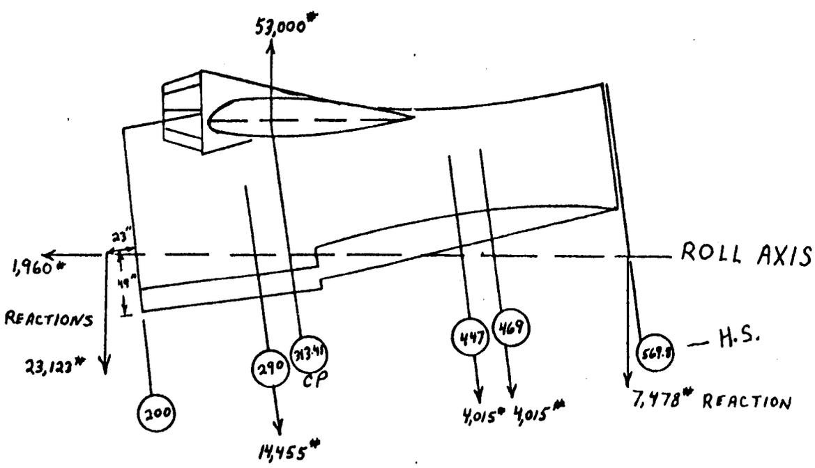
Fig. A-9--Test limit balance loads--positive loading condition
