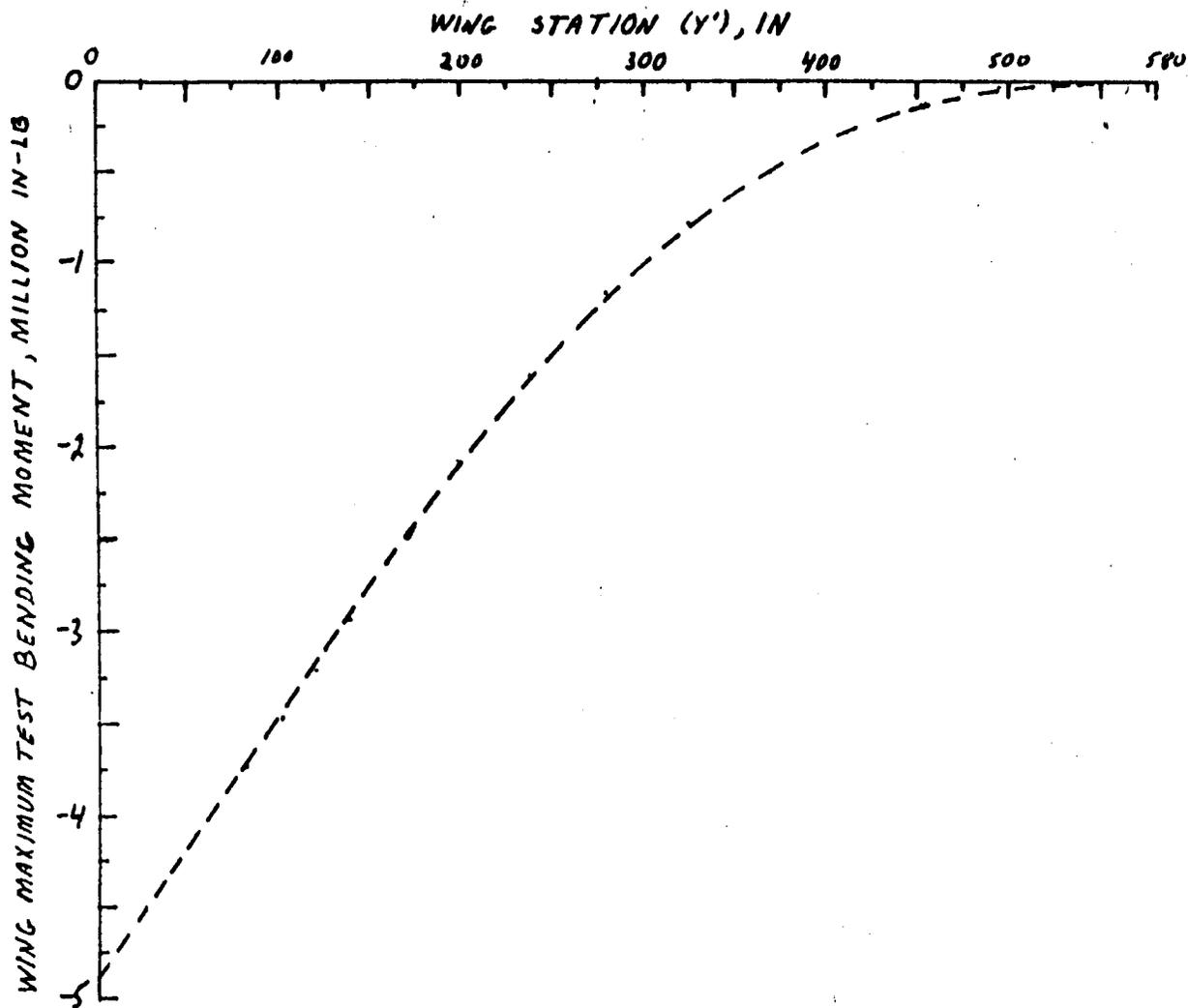
Fig. A-7-- Semispan vertical bending moment distribution--negative loading condition.
