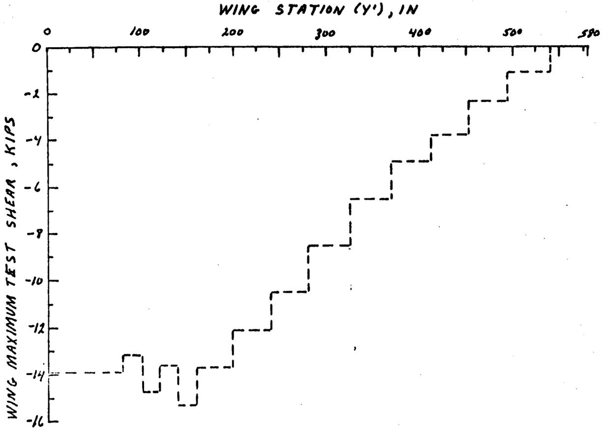
Fig. A-6--Semispan vertical shear distribution--negative loading condition.
