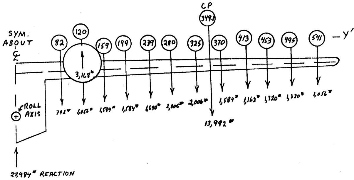
Fig. A-10--Test maximum balance loads--negative loading condition
