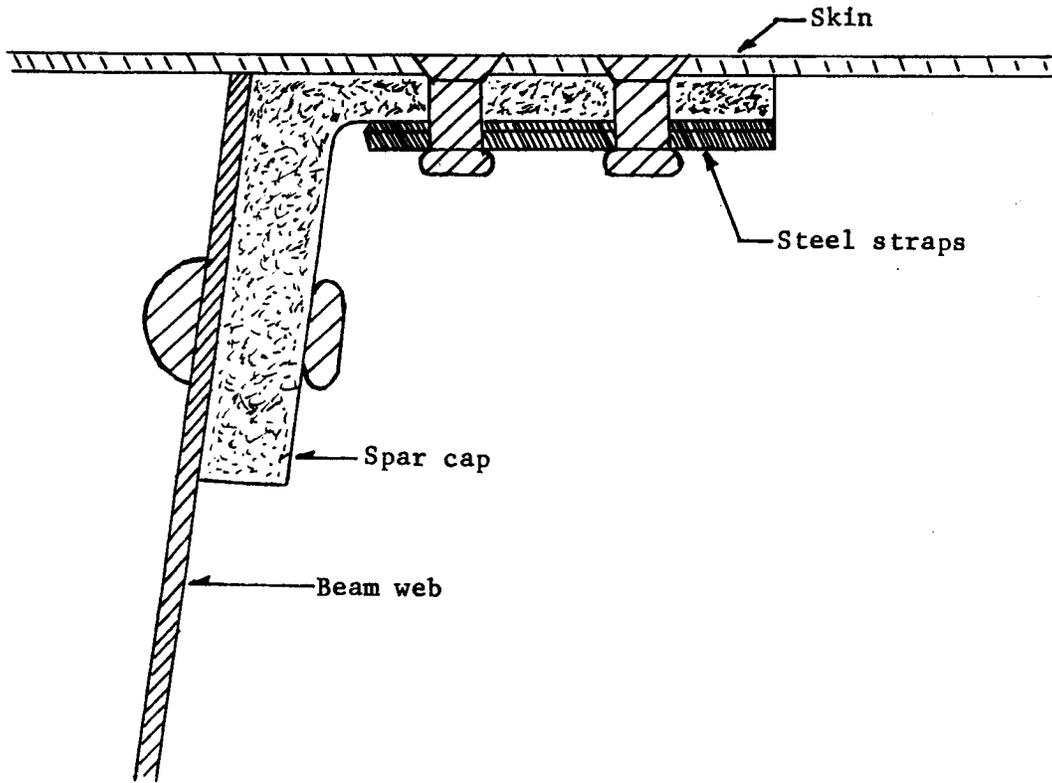
SECTION THRU SPAR CAP
