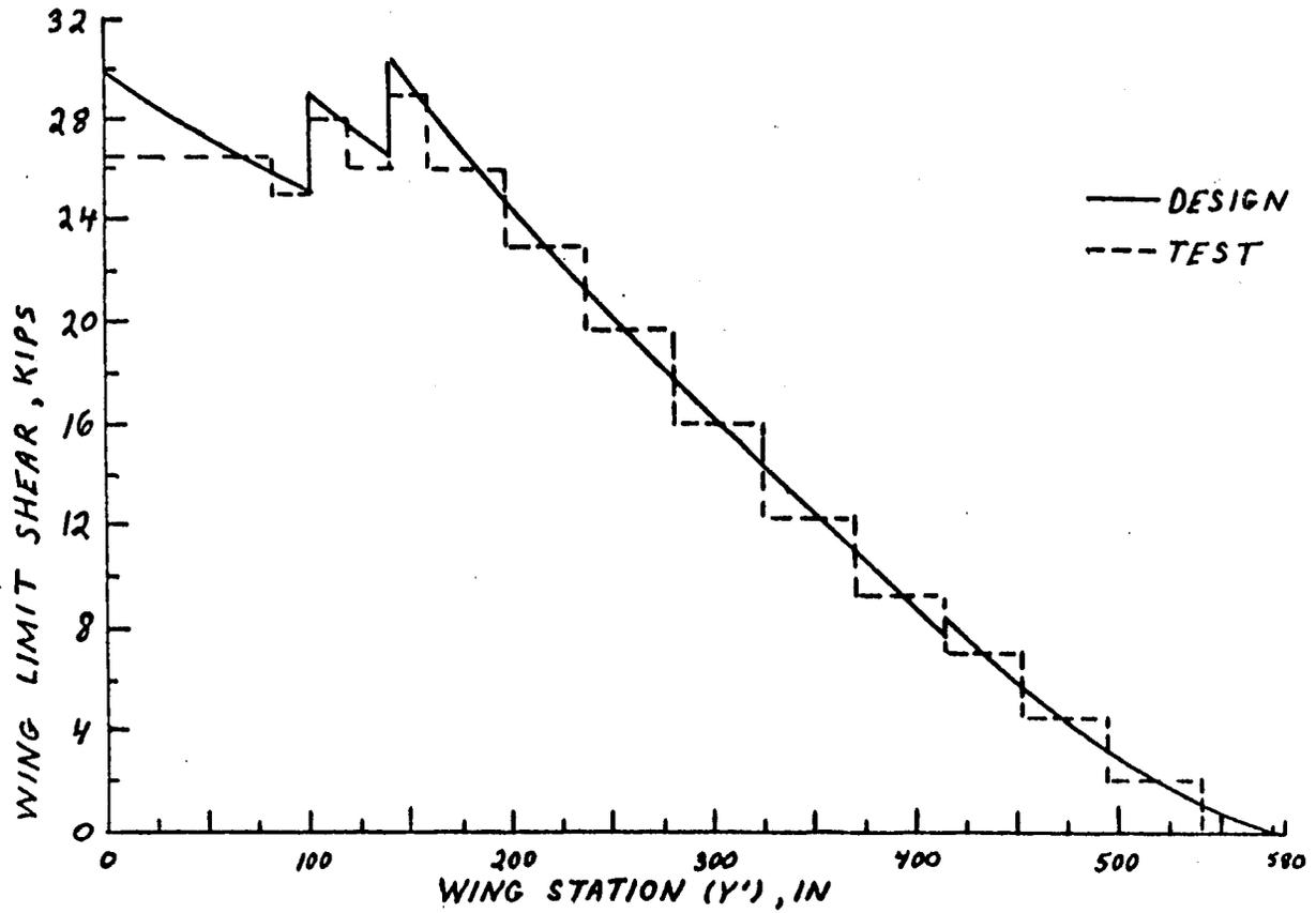
Fig. A-3-- Semispan vertical shear distribution--positive loading condition.
