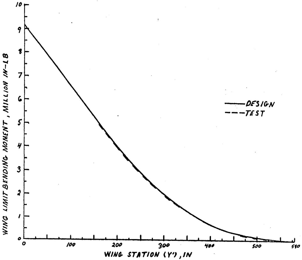
Fig. A-4--Semispan vertical bending moment distribution--positive loading condition.
