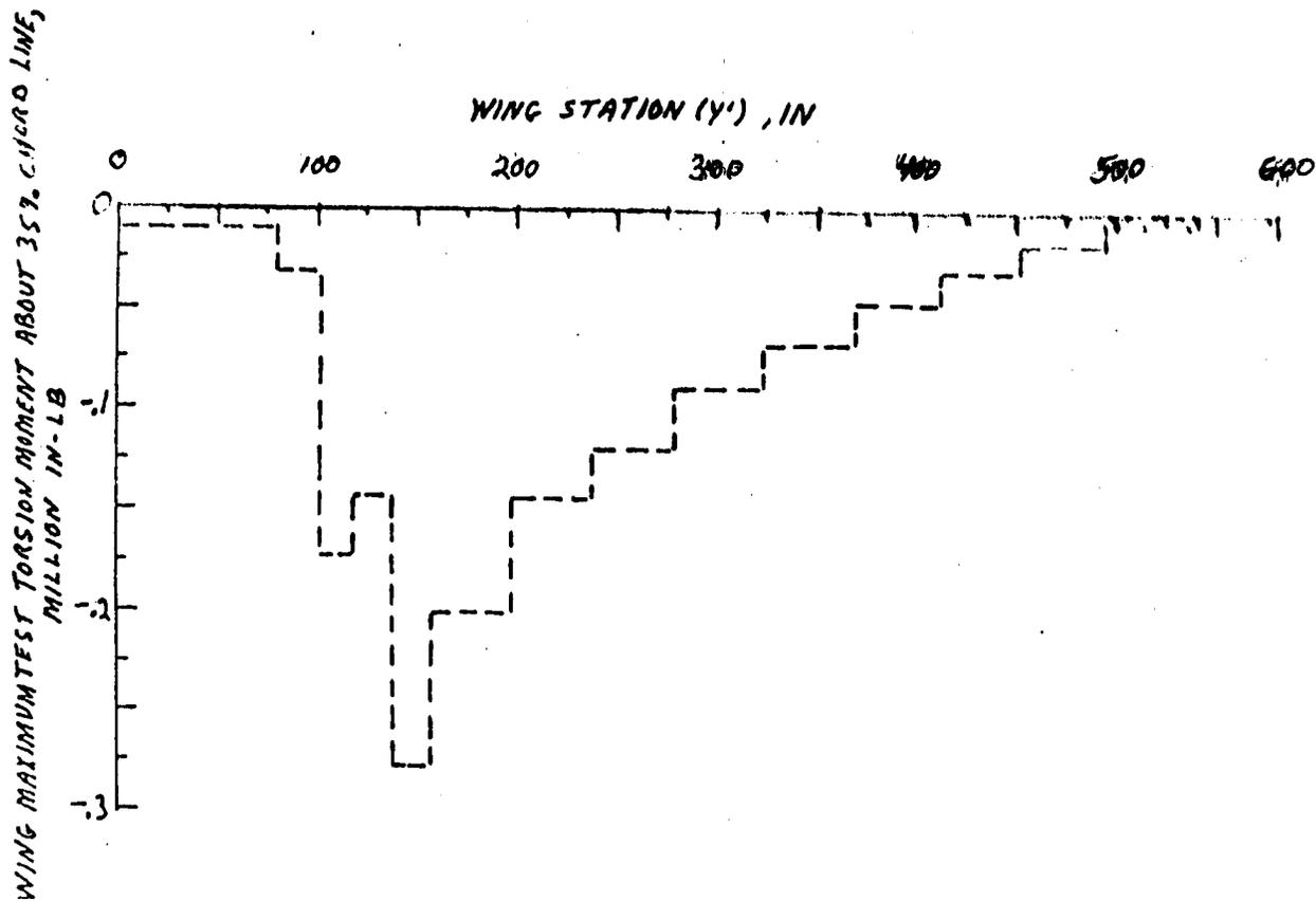
Fig. A-8--Semispan torsional moment distribution--negative loading condition.
