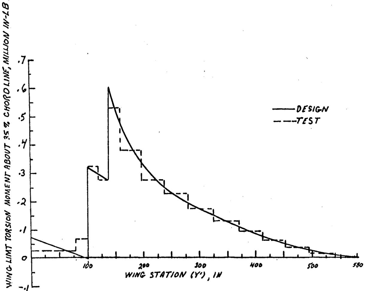
Fig. A-5--Semispan torsional moment distribution--positive loading condition.
